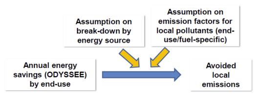
Figure 1: Schematic process of the calculation of avoided local emissions
